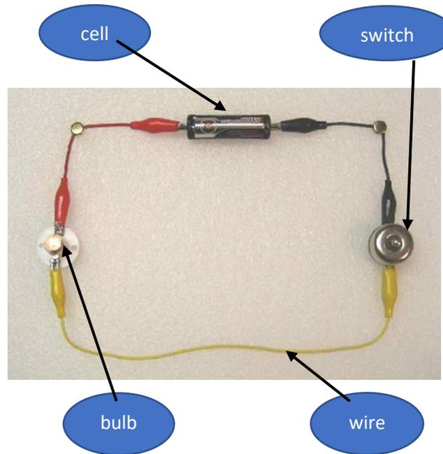
The switch opens and closes the circuit. The bulb lights in this circuit because the switch is on.
